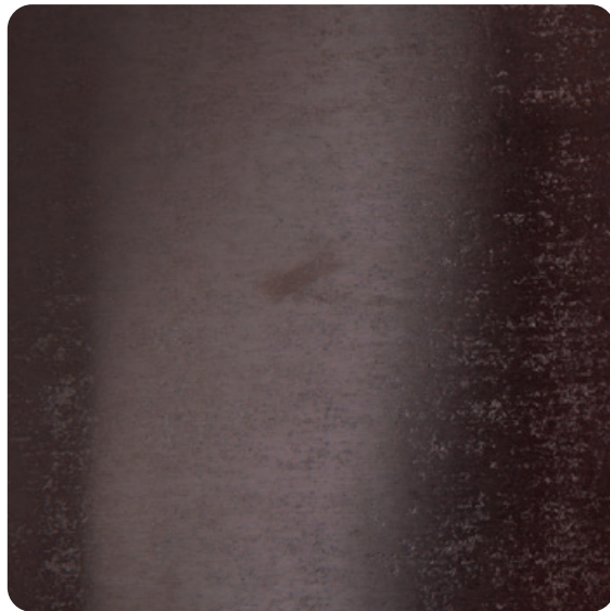
Burnout due to a defect of the outer layer (stain from grinding)
