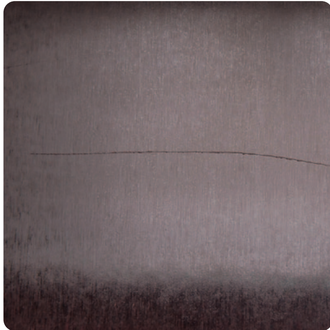
Scratch damaging the laminated coating
