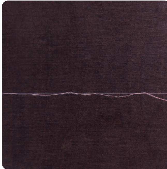
Scratch damaging the laminated coating
