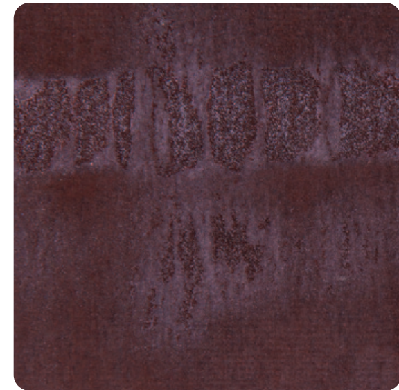
Burnout due to a defect of the outer layer (stripe from grinding)
