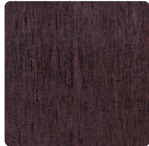
Coverage of wood structure after grinding
