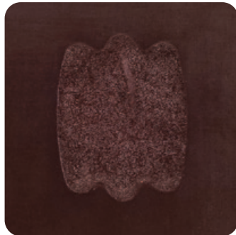
Burnout due to a defect of the outer layer (an insert fallen out)
