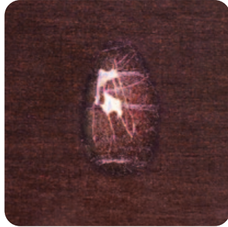
Burnout due to a defect of the outer layer (an insert fallen out)
