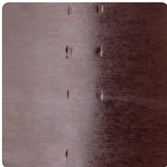
Dent (made by conveyor chains)
