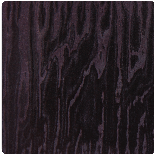
Temperature stains with integrity damage of laminated coating
